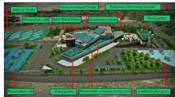
Fig. 2. Introducing the systems used in this project (6)
