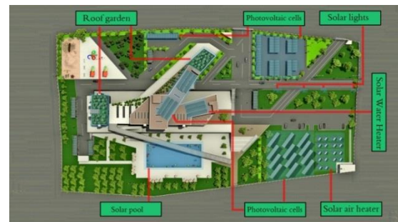
Fig. 1. Introducing the systems used in this project
