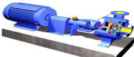
Fig. 3. horizontal centrifuge electro-pump with direct coupling to the electromotor.
