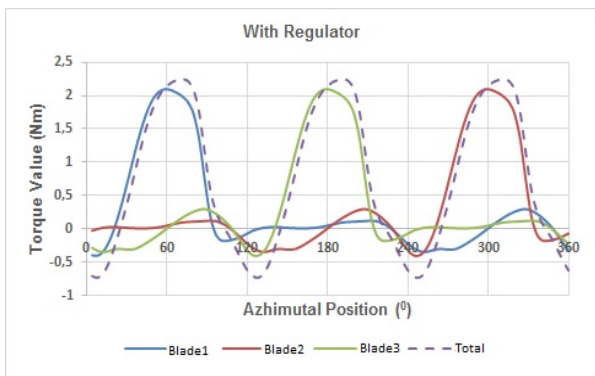
Fig. 4. Torque values as a function of rotor azimuthal position for NACA0015 for with regulator.
