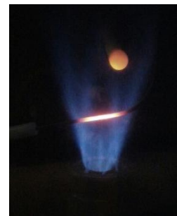
Fig. 9. Flame image of 28% H_2 -52%CO-20% CNG mixture.
