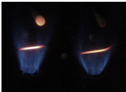
Fig. 7. Flame images of 60% H_2 -20%CO-20% CNG mixture at different swirl numbers: (Left) 0.4, (Right) 0.8.
