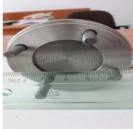
Figure 2. Gas flow plate
