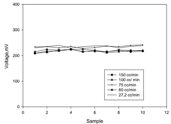
Figure 9. Effects of air flow rates at 700 °C and 25 cc/min hydrogen flow rate
