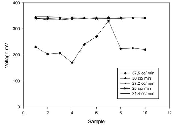
Figure 8. Effects of hydrogen flow rate at 700 °C, and 42.8 cc/min air flow rate
