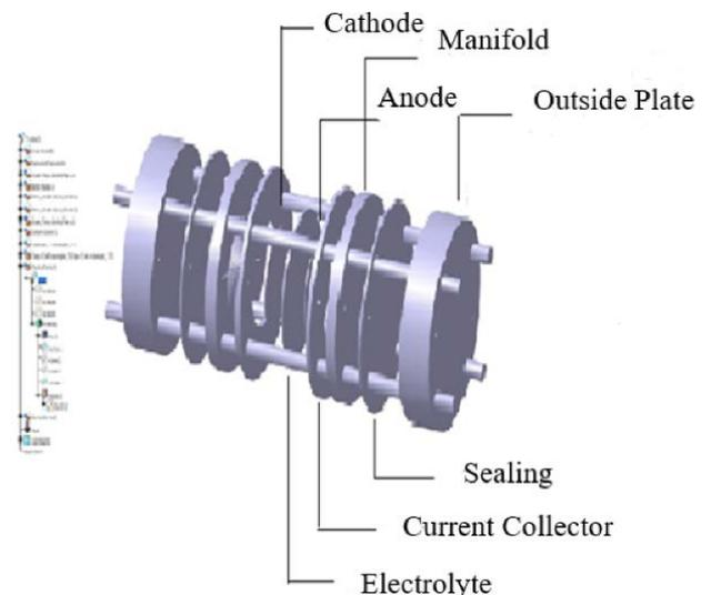
Figure 1 Schematic diagram of MCFC layout with Catia model
