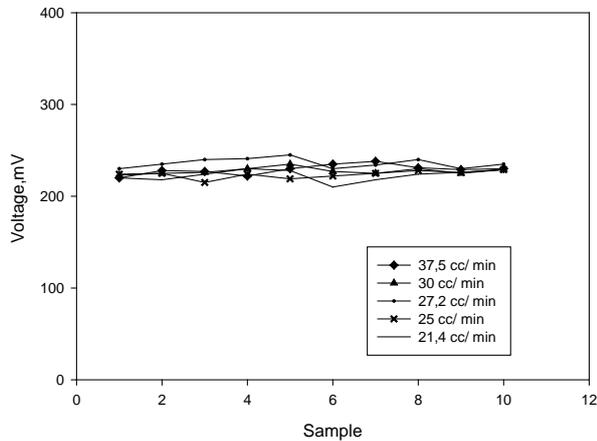
Figure 10. Effects of Hydrogen Flow Rates Diagram at 650 °C and 60 cc/min Air Flow Rate
