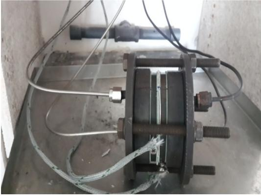
Figure 7. Molten Carbonate Fuel Cell
