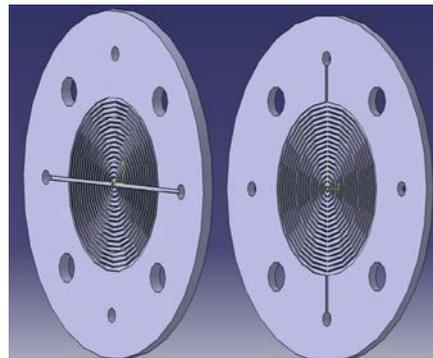
Figure 3. Catia model for the gas flow plate
