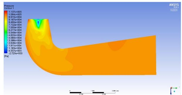
Fig. 10. Pressure distribution of draft tube
