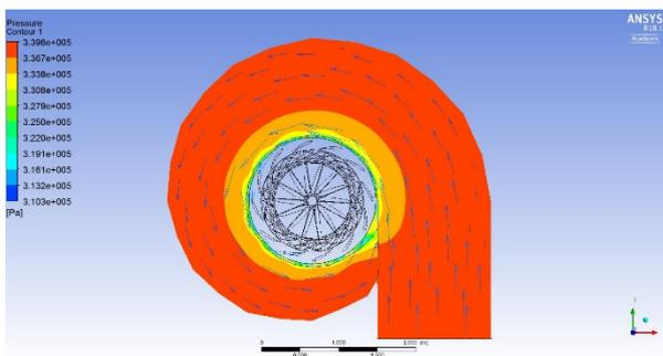
Fig. 7. Pressure distribution and velocity vectors on spiral case
