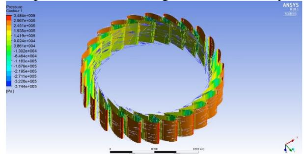
Fig. 8. Pressure distribution and velocity vectors on guide vanes
